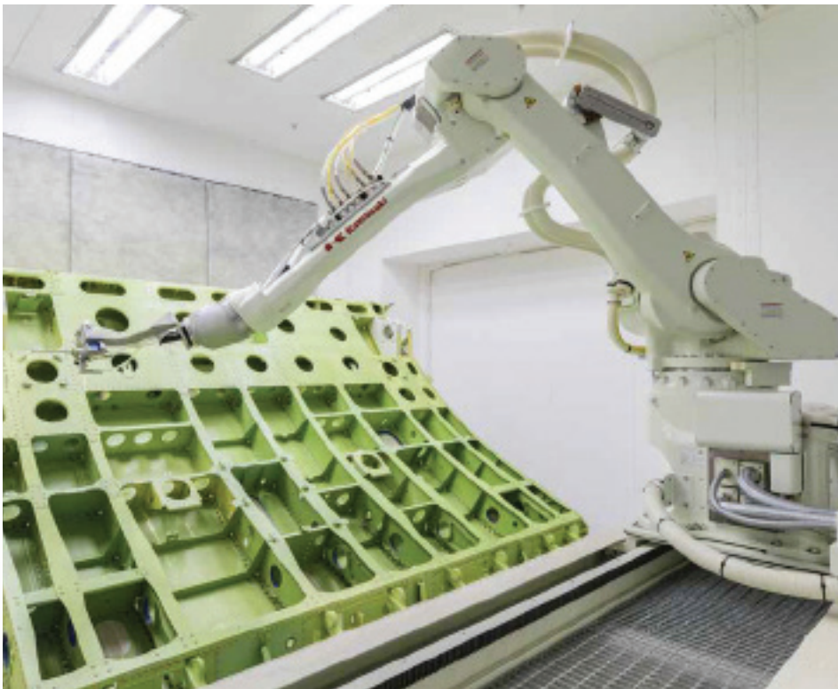
The manufacturing of Boeing 777X cargo doors with Kawasaki's automated manufacturing systems.
