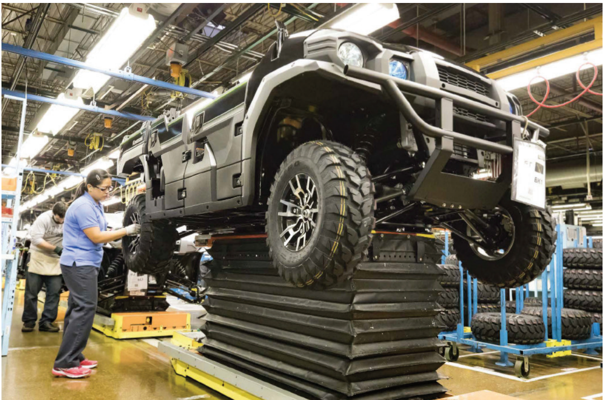
Part of Kawasaki Lincoln's production line for MULE utility vehicles.
