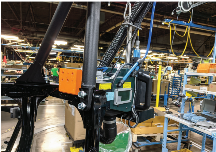
Kawasaki’s laser engraving system etches vehicle identification numbers (VIN) onto vehicle frames with a 3D printed clamp (left).
